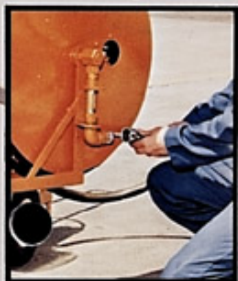
6. Attach hose from pump eductor to hose reel.
