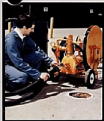
2. Attach quick-coupled hoses to pump suction and discharge.
