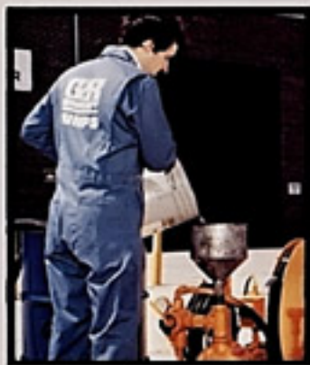
3. Fill volute casing with priming liquid.
